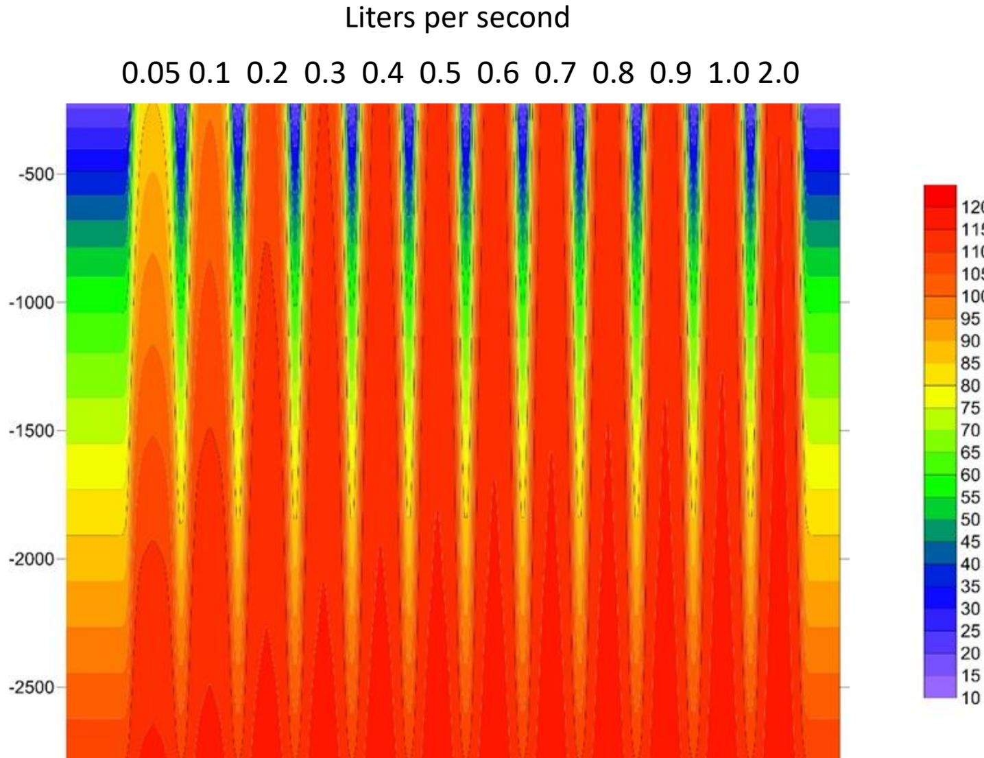
Simulated temperatures in 2-D models in 3-km vertical pipes at different velocities suggest that high formation temperatures reach the surface.
