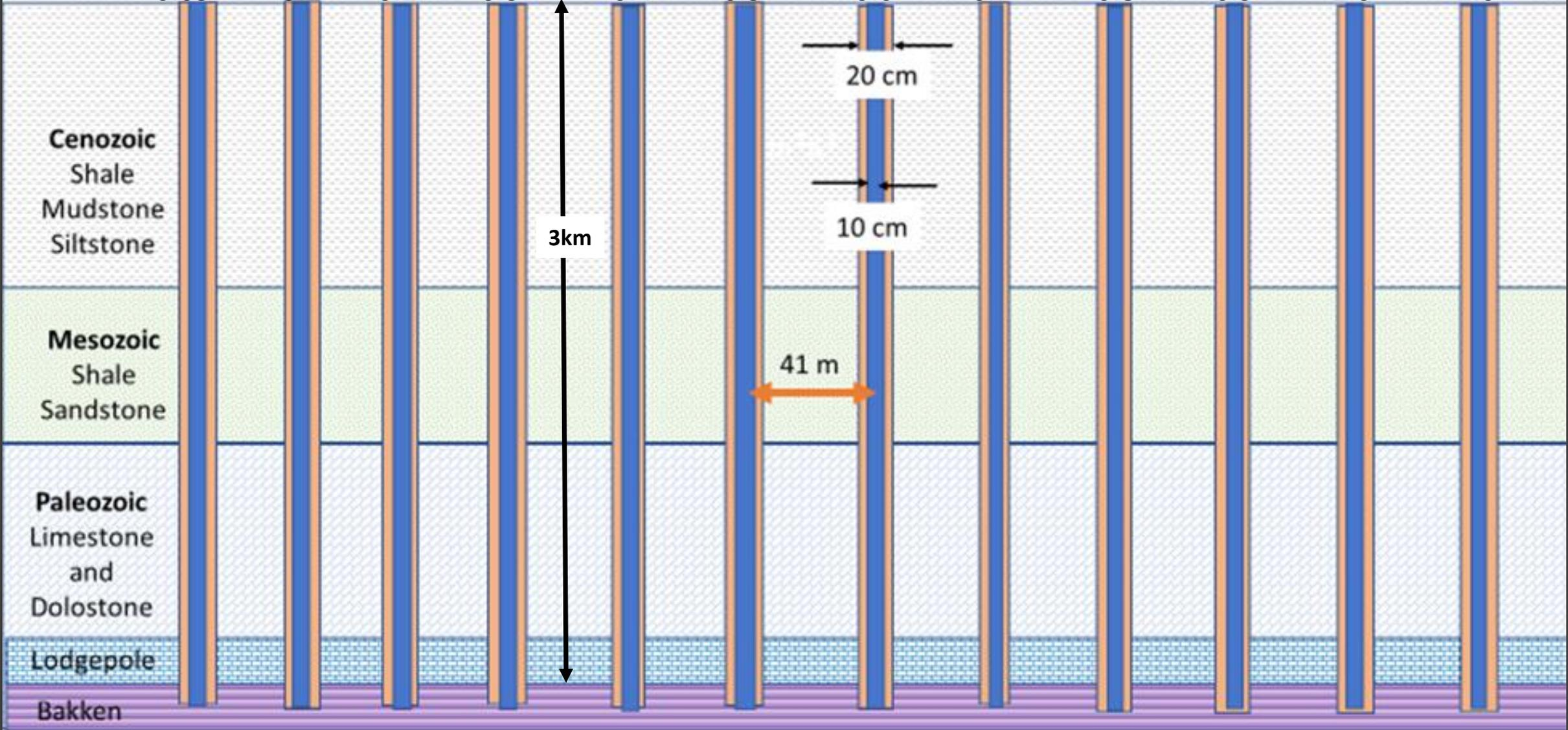
Comparison of heat exchange surfaces in 2-D and 3-D models of fluid flow in vertical wells.
