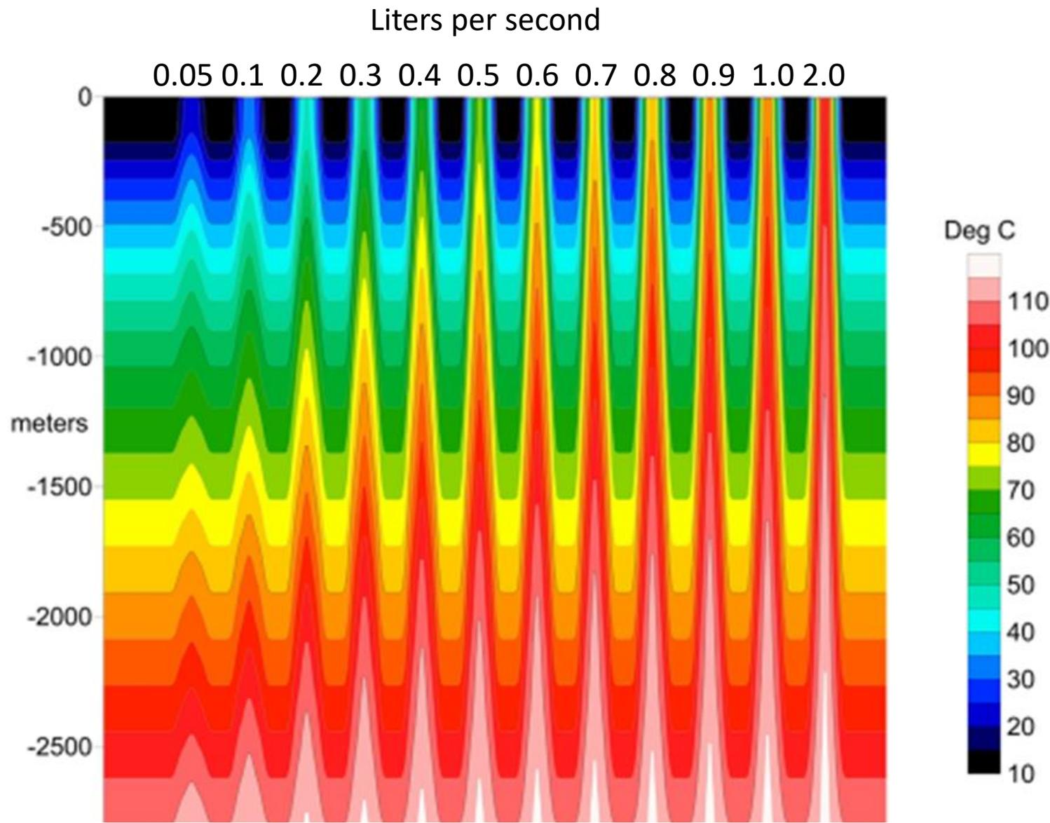
Simulated temperatures in 3-D models in 3-km vertical pipes at show that high formation temperatures do not reach the surface at average Bakken production velocities.
