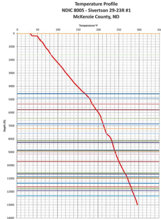
Figure 4: Temperature profile of a well drilled in the Williston Basin in North Dakota. The coloured horizontal lines indicate depths of formation tops. The profile is from a continuously logged well bore and shows fluctuations in slope (temperature gradient) as well as smaller and more localized inflections downhole between formations with differing thermal conductivities (McDonald, 2015).
